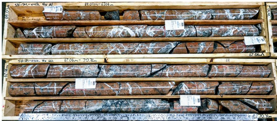
**Photo 2.** Mineralization encountered in drillhole SH21-042 from 64.0 – 70.3 m; preliminary assay results for 65.5 m to 67.0 m: 1.42 g/t Au and 67 g/t Ag [2.25 g/t AuEq\*].
