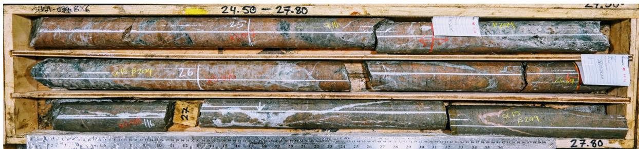
**Photo 1.** Mineralization encountered in drillhole SH21-039 from 24.5 – 27.8 m; preliminary assay results for 25.4 m to 26.7 m: **1.70 g/t Au and 96 g/t Ag [2.90 g/t AuEq\*]**.
